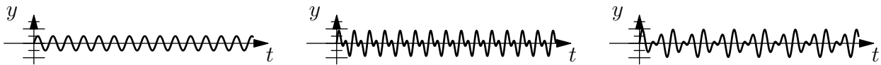
Figure 1: A pure sine wave, a pure sine wave played with the octave above it, and a pure sine wave played with the perfect fifth above it.
